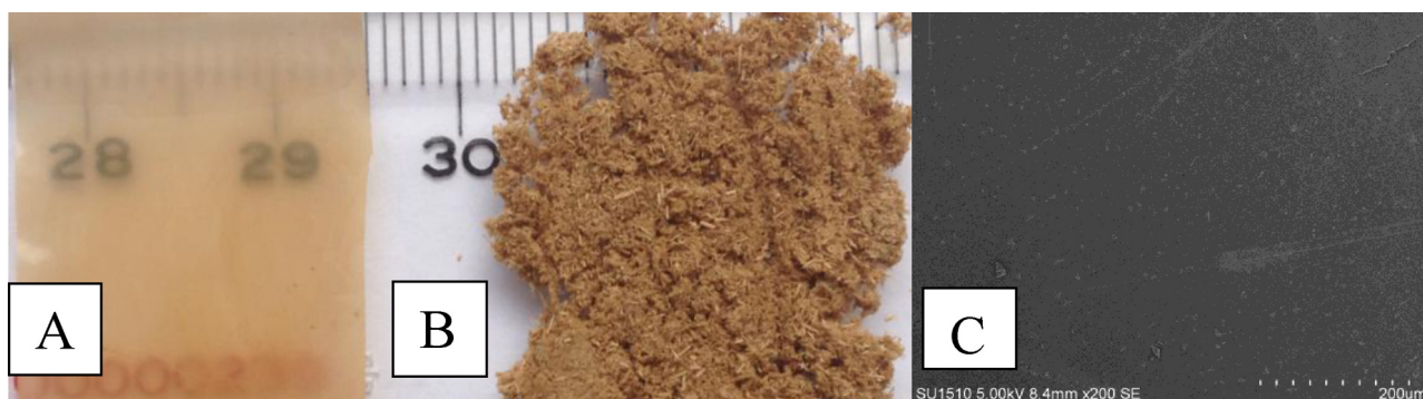
Fig. 9. Digital photo of the acetylated RS (WPG = 35.5%) film (A) and RS (B) with 20% DEP, respectively, and SEM (C) of the acetylated RS (WPG = 35.5%) film with 20% DEP.
